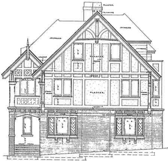
Front elevation and first floor plan of George Chambers house on Santa Rosa Avenue, 1908, dating from Morgan's early partnership with Ira Hoover. Half timbering, brick veneer, and leaded glass are indicated on elevation; plan shows typical symmetry of front rooms and hall, side entry, and small kitchen, pantry, and maid's room. Three-story house has 7 bedrooms. (Lynn Stone collection)
